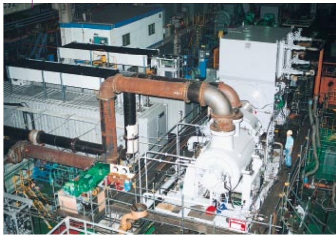
BCH804 Complete Unit Test with 35MW Motor
