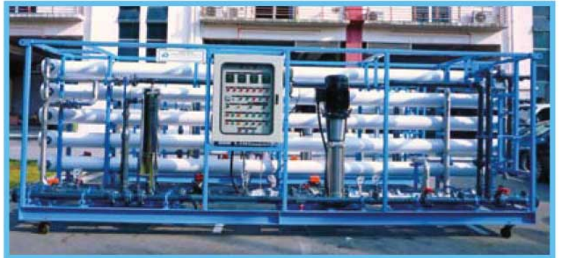
500,000 litres/day production capacity MBR-RO in Abu Dhabi, UAE
