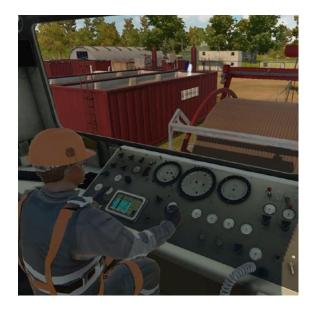
Valve alignment, for both suction and discharge of the fluid pump system are all selected by the student at the student input station. Students are required to select fluid type and density and to monitor the transfer of fluids from and to the mixing tank.
